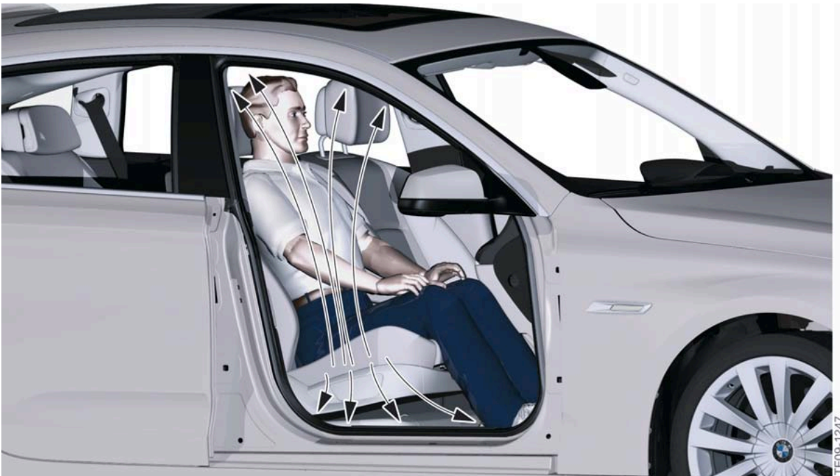
Measuring procedure of the CIS mat, example: F07
